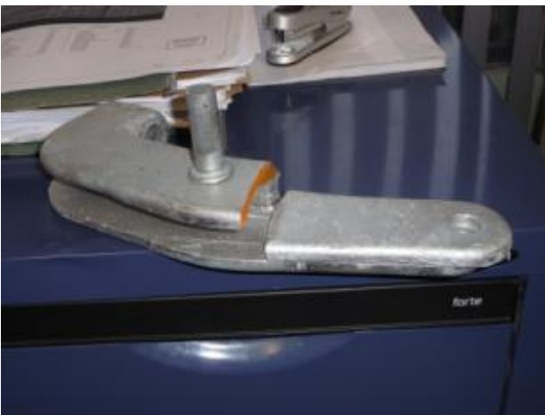
Figure 14: Example of fractured banana end of proprietary brace connector in the roof plane of a long span steel portal frame building From left to right: (a) Global view; (b) Close-up view. [Photos by M. Bruneau].
