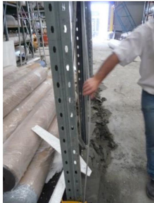
Figure 16: Industrial storage racks that survived, with evidence of soil liquefaction From left to right; (a) Global view; (b) Close -up of buckled brace. [Photos by M. Bruneau].
