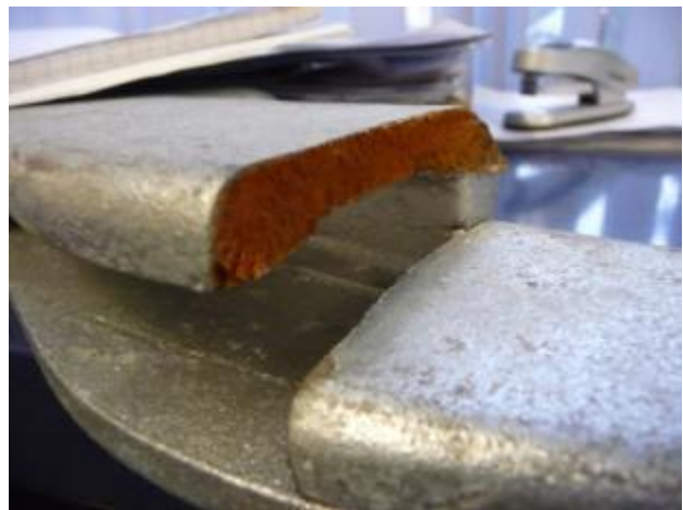
Figure 14: Example of fractured banana end of proprietary brace connector in the roof plane of a long span steel portal frame building From left to right: (a) Global view; (b) Close-up view. [Photos by M. Bruneau].
